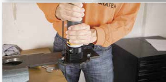
Initial drill holes from: Ø 3.0 mm for pin cutters Ø 5.0 mm in spherical cutters
