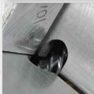
Precise deburring by rolling milling
