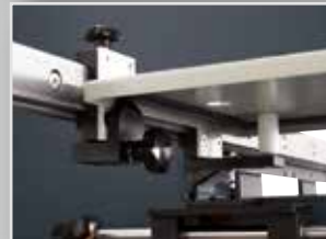
Reciprocal quick-clamping system for edge folds either top or bottom
