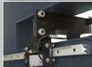
Path measurement of X and Y travel
