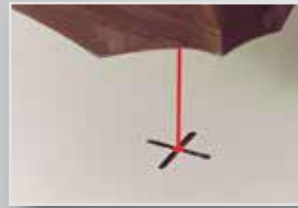
Laser pointer for optical display of tool centre
