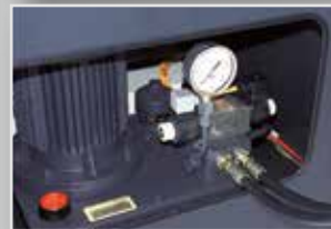
Dual-circuit hydraulic unit in cabinet base
