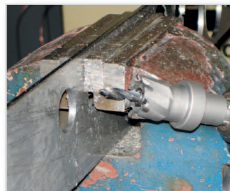
Free-hand drilling up to Ø 30 mm
