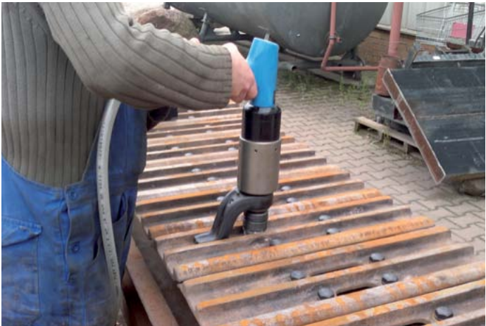
Quiet and accurate torque - even from just 2 bar operating pressure
